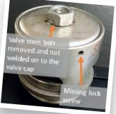
thread inside the nut, preventing the vacuum relief part of the valve from closing.
